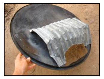
After some experimentation making charcoal with this kiln, a tin baffle was attached with rivets to the inside of the lid. This directed the airflow during the burn to the sides of the kiln to promote more consistent pyrolysis within the different zones inside the kiln.
