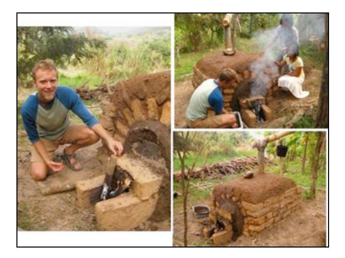
Note the bucket attached to the bamboo chimney for collection of wood distillates (pyroligneous acid, or wood vinegar).
