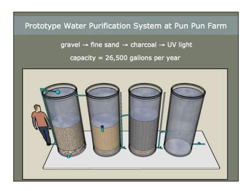
Here's an illustration done by my colleague of how the system will be configured, with gravel and sand filters to remove turbidity and microorganisms, and an optional germicidal UV unit for further disinfection
