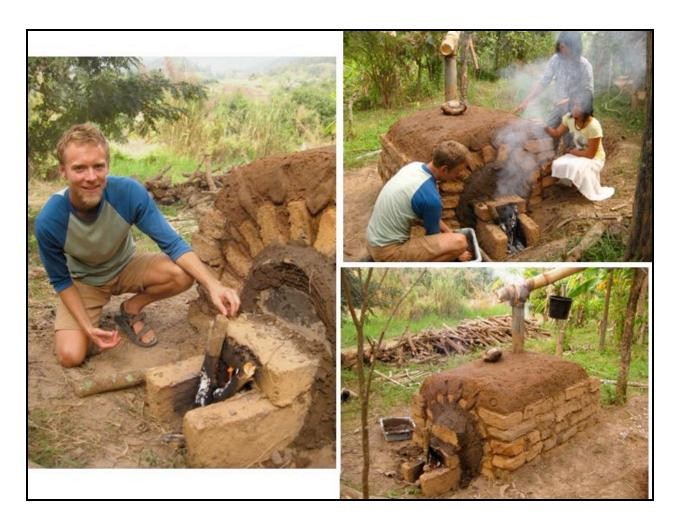
Note the bucket attached to the bamboo chimney for collection of wood distillates (pyroligneous acid, or wood vinegar).
