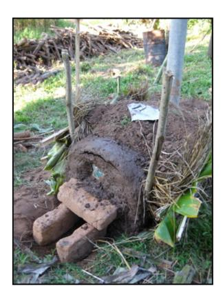
An inlet is made with adobe bricks, and the lid plastered with mud for insulation and to seal the kiln.
