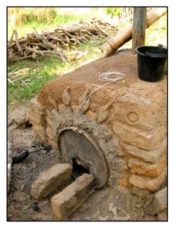
A thermocouple probe (K-type) was inserted into the kiln and connected to a temperature datalogger. The tip of the probe was placed as near to the center of the kiln as possible.
